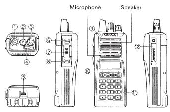
Note: The transceiver is also available without the DTMF keypad (①).
