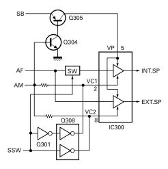
Fig. 4 Audio amplifier circuit
