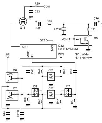
Fig. 3 Wide/Narrow changeover circuit
