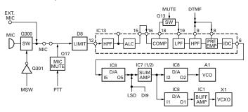
Fig. 7 Microphone amplifier
