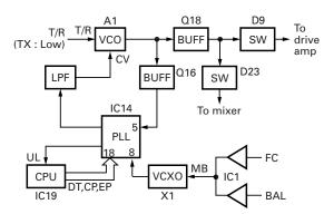
Fig. 9 PLL block diagram
