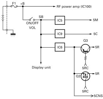
Fig. 15 Power supply circuit
