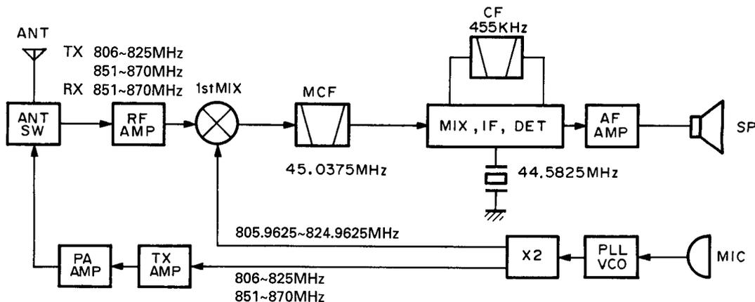
Fig. 1 Frequency configuration
