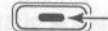
Lights green while the preamp is activated; lights red while the attenuator is activated.
