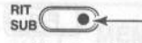
Lights red while the RIT function is activated; green while the SUB DIAL function is activated.
