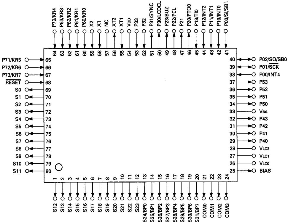
**Microprocessor : μPD78310AGF (TX-RX unit IC4)**
