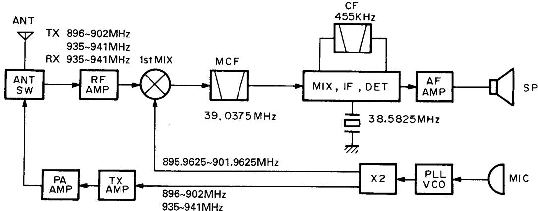
Fig. 1 Frequency configuration
