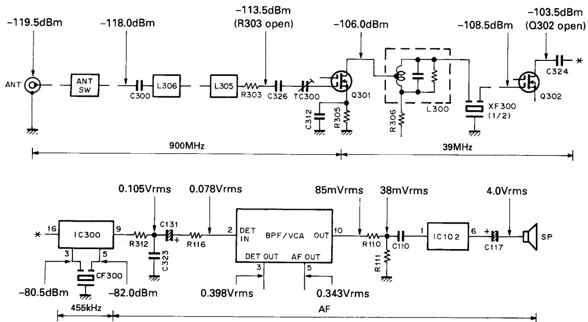
To make measurements in the AF section, connect the oscilloscope probes directly.
