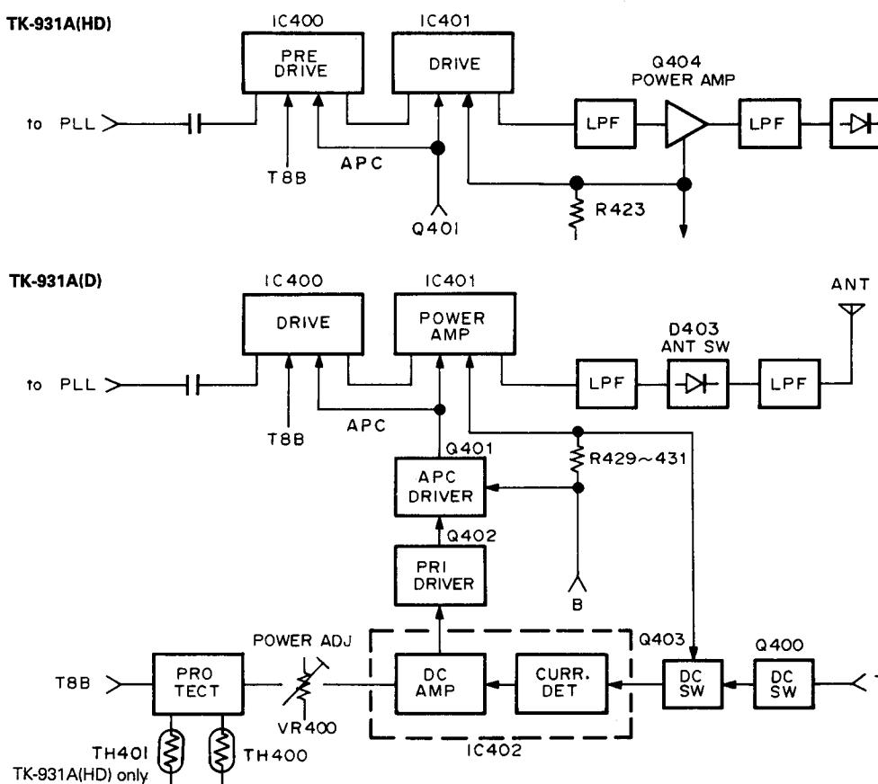
Fig. 5 Transmit power unit, APC circuit
