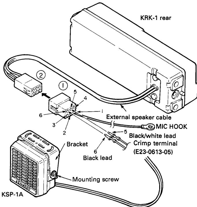
4. Connection of TK-931A(D)/931A(HD) remote unit.
