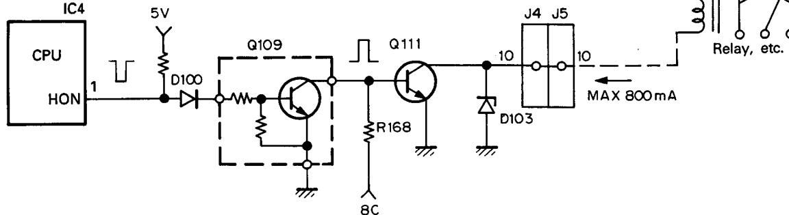
Fig. 11 Horn control circuit
