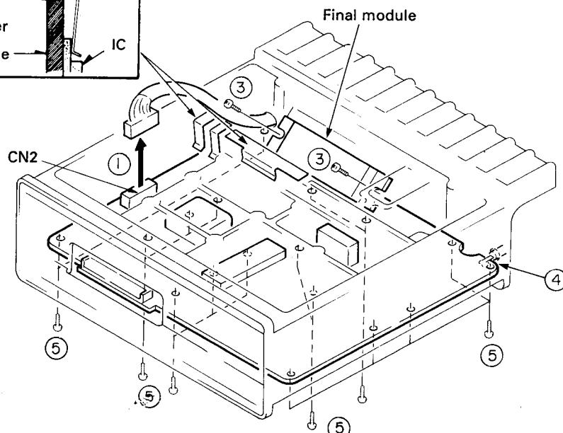
**Note :** To replace the final module, remove the lead soldered to the TX-RX unit.
