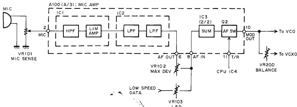
Fig. 4 Microphone amplification
