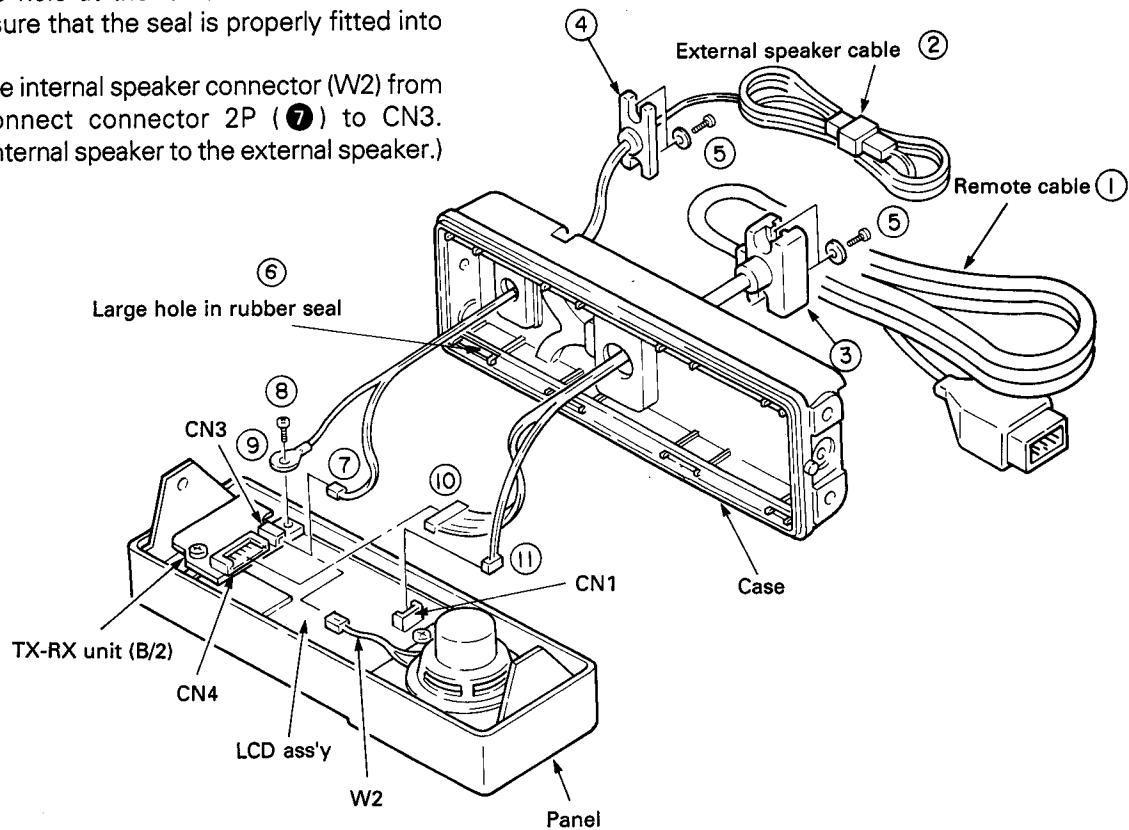
9. After inserting the connectors into the panel, secure the harness with the two supplied nylon bands (12 and 13) over the center line of the panel.
