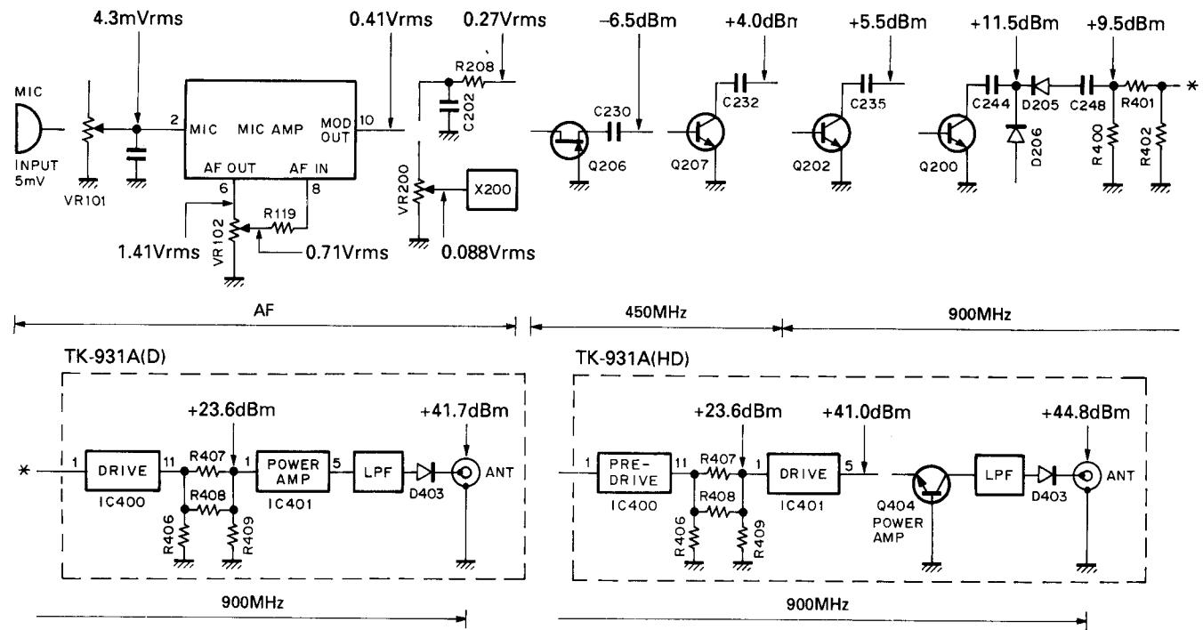
To make measurements in the AF section, connect the oscilloscope probes directly.
