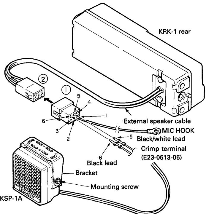
4. Connection of TK-930A(D)/930A(HD) remote unit.
