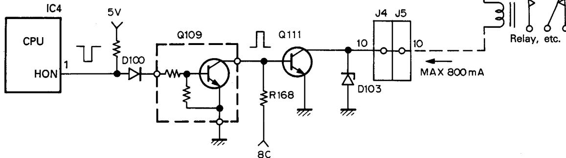
**Fig. 11 Horn control circuit**
