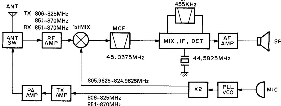
**Fig. 1 Frequency configuration**
