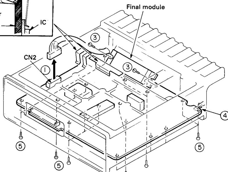
**Note :** To replace the final module, remove the lead soldered to the TX-RX unit.
