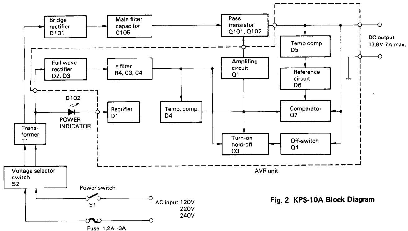
Fig. 2 KPS-10A Block Diagram
